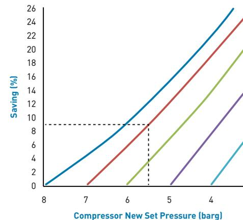
For example, energy consumption can be reduced by 9%, when air set pressure is reduced from 7 barg to 5.5 barg. It means 5000 Euro can be saved annually for 100 kW power compressor.
