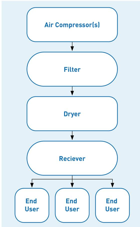
Compressed air systems consist generally of the following main parts.
